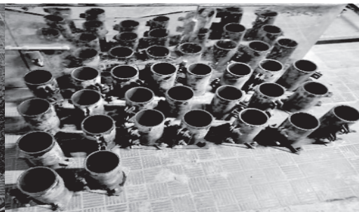
Fig. 4: Mold Ready for Casting.
